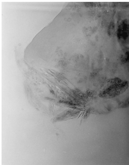
Fig. 5. TEM of (Mg/G) BN with magnifications of 2 \times 10^5 . (Mg/G) BN was prepared by grinding of Mg (4.2 g) and graphite (1.8 g) with benzene (8 cm 3 ) for 25 h.
